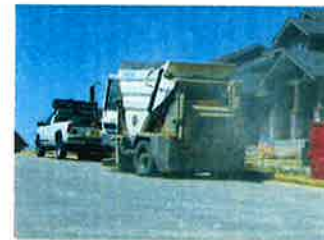
Photograph SS-1. A street sweeper removes sediment and potential pollutants along the curb line at a construction site. Photo courtesy of Tom Givie.
