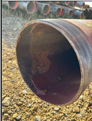
5. Column Pipe - Interior Pitting
