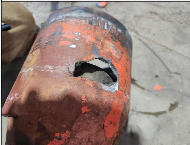
4. Swage Nipple Corrosion
