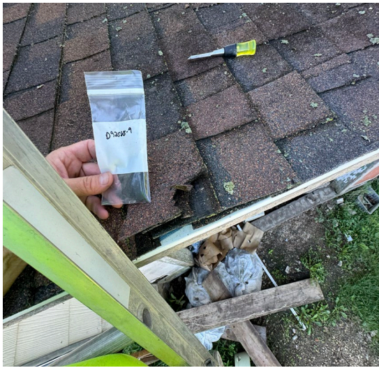
Sample D92525-9: Singles/ice dam on roof negative for asbestos.
