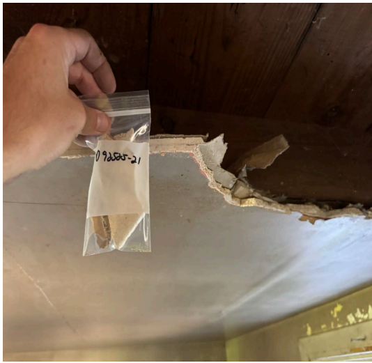
Sample D92525-21: Plaster/drywall backer in kitchen ceiling negative for asbestos.
