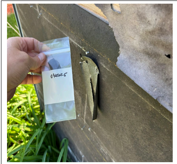
Sample D92525-5: Tar strips behind siding negative for asbestos.
