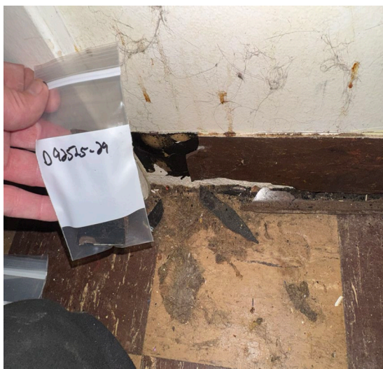
Sample D92525-29: Base cove/adhesive end floor bedroom negative for asbestos.
