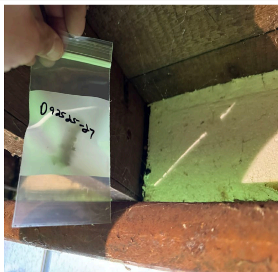
Sample D92525-27: Black caulking in the basement, rim joist, positive for asbestos.
