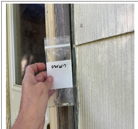
Samples D92525-7: Caulking around exterior windows negative for asbestos.
