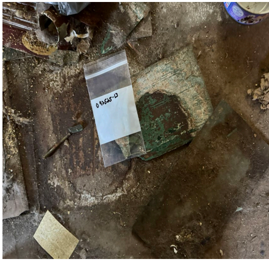
Sample D92525-13: Floor tile positive for asbestos, throughout first floor (Mastic PC less than <1%)
