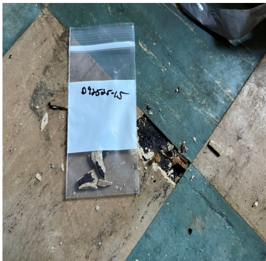
Sample D92525-15: Floor tile positive for asbestos, throughout first floor (Mastic PC less than <1%)
