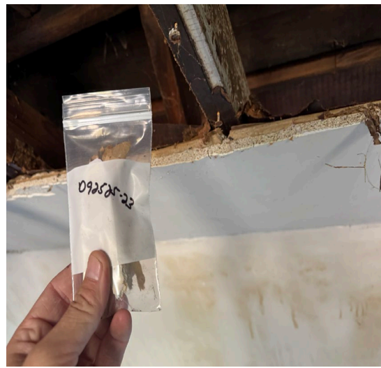
Sample D92525-22: Plaster/drywall backer basement landing <1% asbestos (PC).
