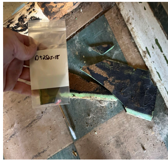
Sample D92525-18: Vinyl base/adhesive in main room negative for asbestos.
