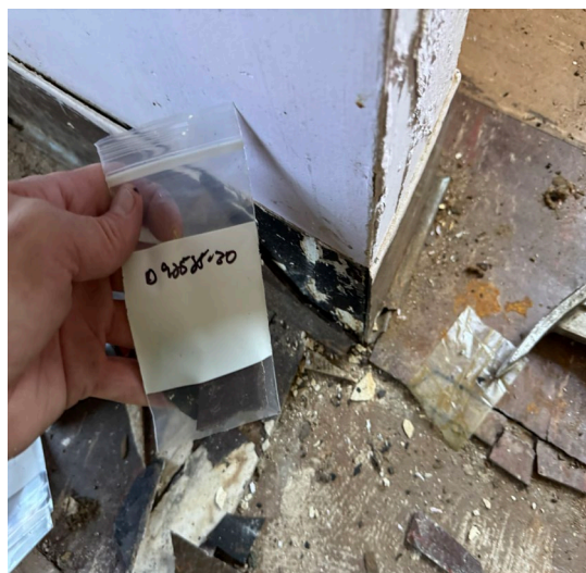
Sample D92525-30: Base cove/adhesive end floor bedroom negative for asbestos.
