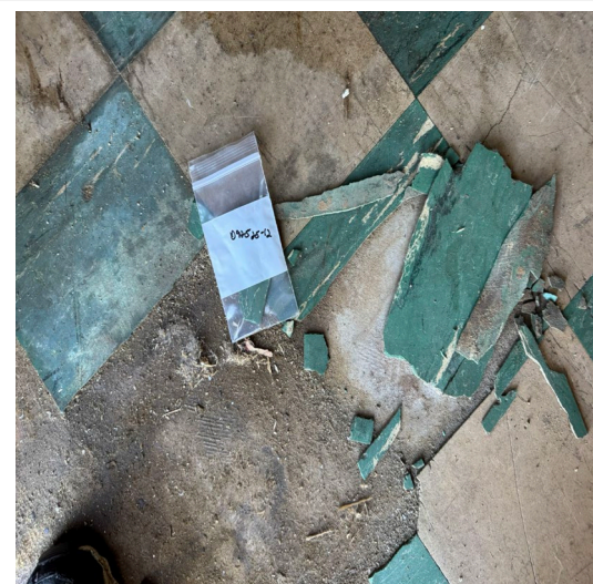
Sample D92525-12: Floor tile positive for asbestos, throughout first floor (Mastic PC less than <1%)
