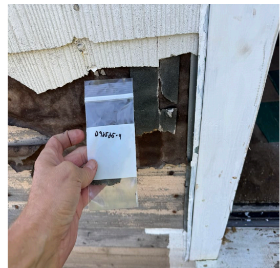
Sample D92525-4: Tar strips behind siding negative for asbestos.
