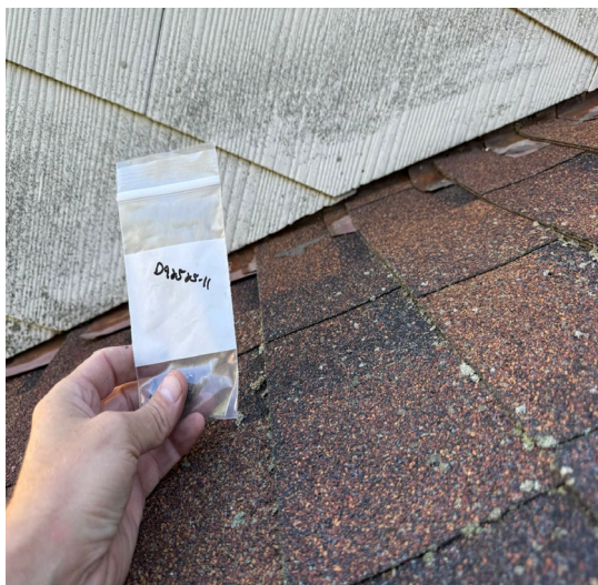
Sample D92525-11: Tar on roof negative for asbestos.
