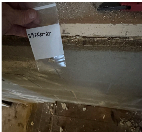
Sample D92525-25: Caulking, White, at rim joist in basement negative for asbestos.
