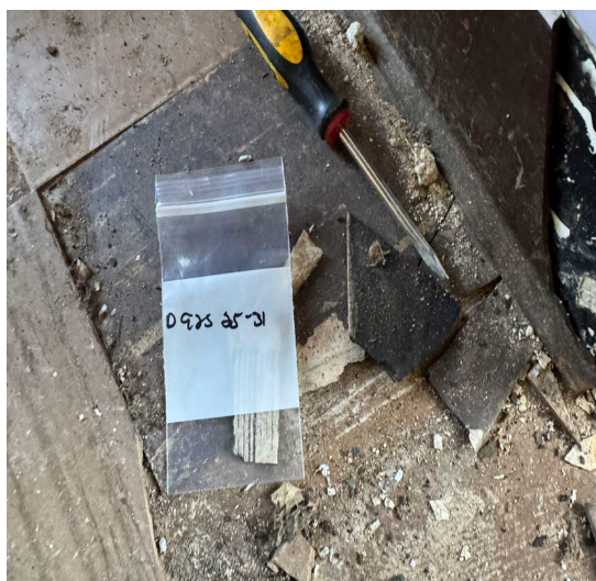
Sample D92525-31: Floor tile 2 nd floor positive for asbestos.
