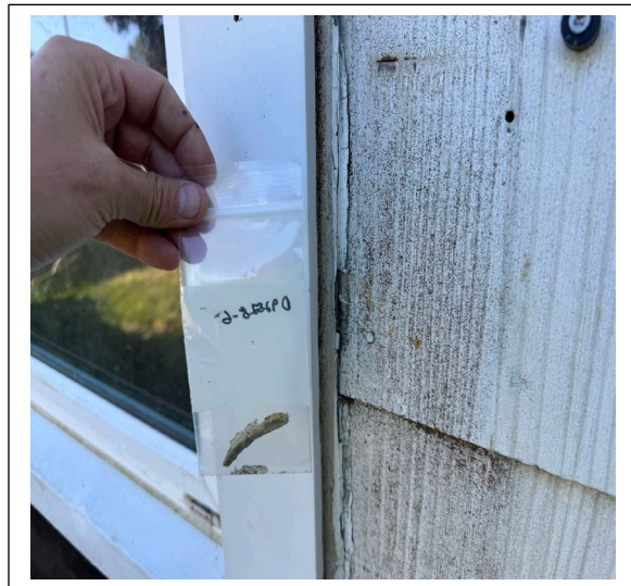
Samples D92525-6: Caulking around exterior windows negative for asbestos.
