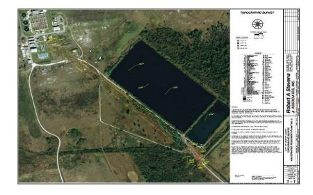
**City of Winter Haven** Wastewater Treatment Plant **No. 3 Outfall Improvements** This project included a topographic survey of a 3,000+ foot corridor and adjacent pond area for rerouting the processed water outfall from Wastewater Treatment Plant No. 3 to interconnect with the existing swale crossing the CSX Intermodal property. Team Members: Robert Stevens, Matthew Stevens, Andrew Stevens **Project Value:** \$6,475 **Completion Date: 2011**
