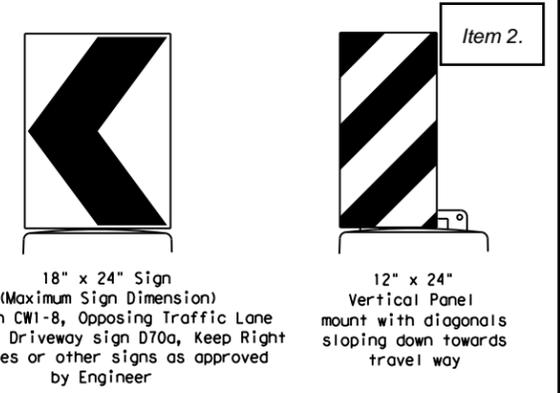
Plywood, Aluminum or Metal sign substrates shall NOT be used on plastic drums
