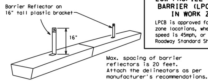
**LOW PROFILE CONCRETE BARRIER (LPCB) USED IN WORK ZONES**
