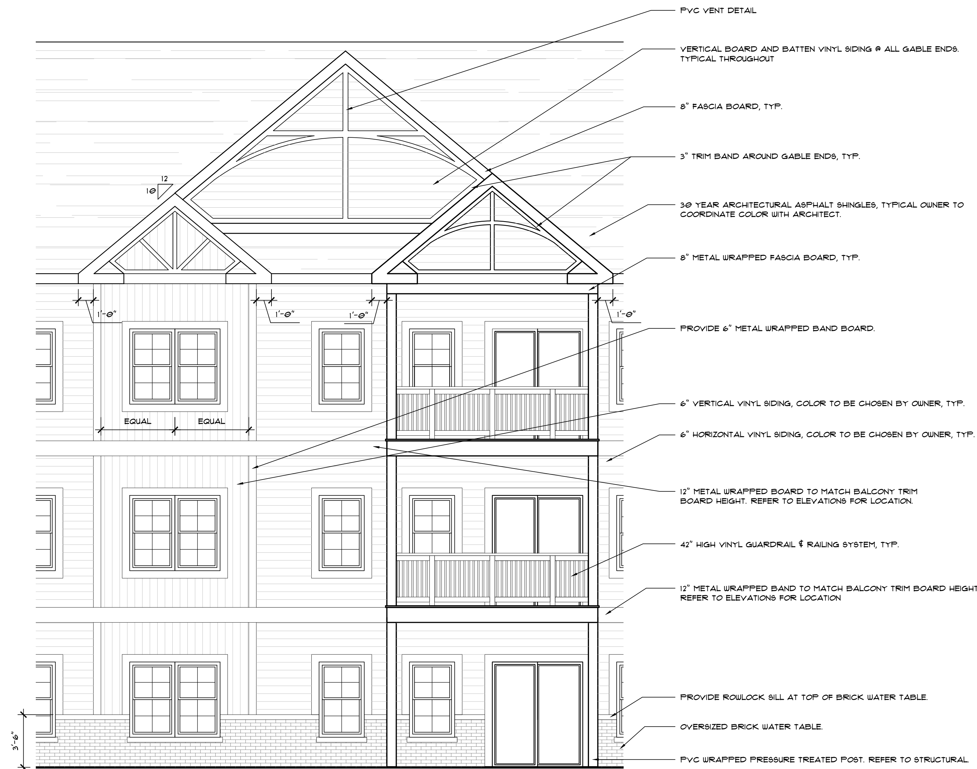
1 ELEVATION DETAIL: REAR GABLE GROUP SCALE: 1/4" = 1'-0"
