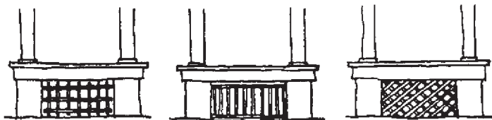
Lattice Infill At Porch Piers
