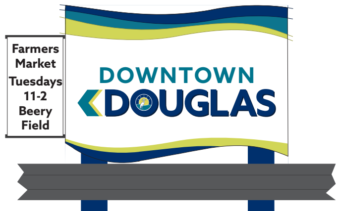
Concept 4 - Sign approximately 106"Wx72"Hx12"D, letter height - 12.6"H Side banner brackets for event advertisements.
