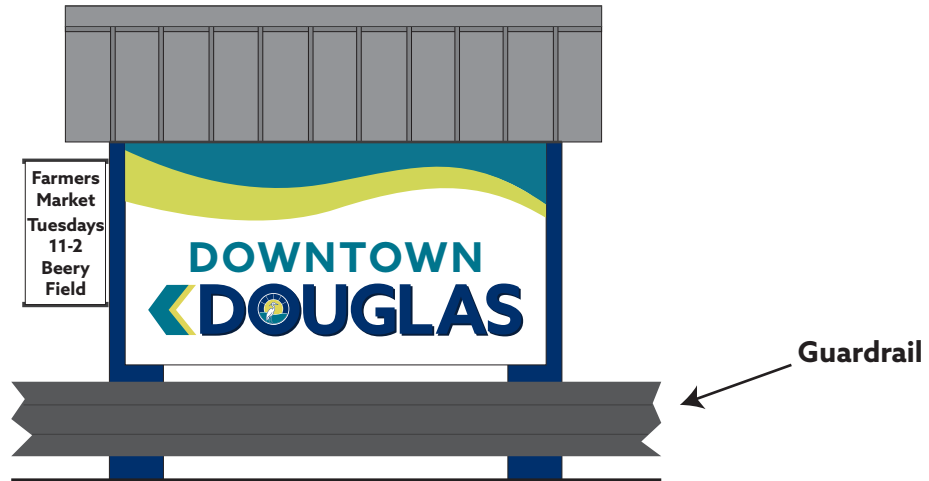
Concept 1 - Sign is approximately 93.5"Wx49.5"H, letter height - 11.7"H Use existing structure, redesign sign only using metal, paint main body the dark blue, add banner brackets to left side for event advertisement
