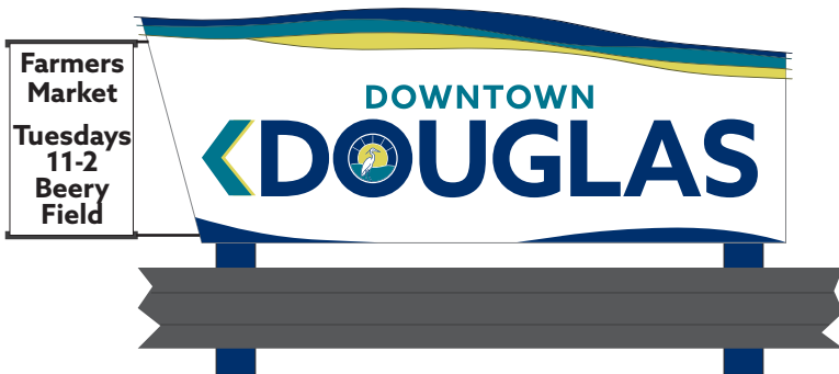
Concept 3 - Sign is approximately 135"Wx48"Hx12"D, letter height - 16"H Copy Center and BSH Gateway shape, back lighting, side banner
