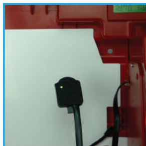
Sensor monitoring the presence of the AED and controlling the temperature
