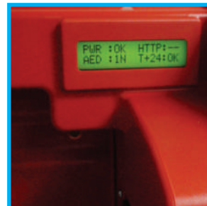
LCD screen displaying general status or incidents
