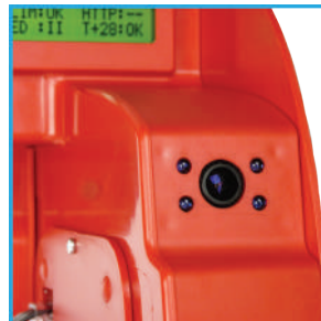
Infra-red lens taking pictures upon the opening of the cabinet and removal of the AED
