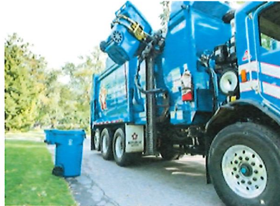
Figure 11. Automated Side Load Collection. Provides a cleaner, safer, more efficient residential collection.
