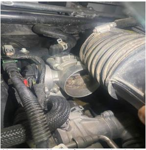
A patrol car suffered engine problems and would not go faster than 10 mph. It was taken to the City Shop where the mechanic found the cause of the problem. A fat mouse had crawled into engine, died, and its body was preventing a valve from fully closing. The mechanic posted the photos on a Ford blog sight and the post went viral.
