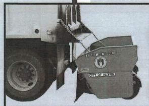
Towed- road speed related Contractor Grade Spreads when driving forward (only) Optional hopper empty sensor
