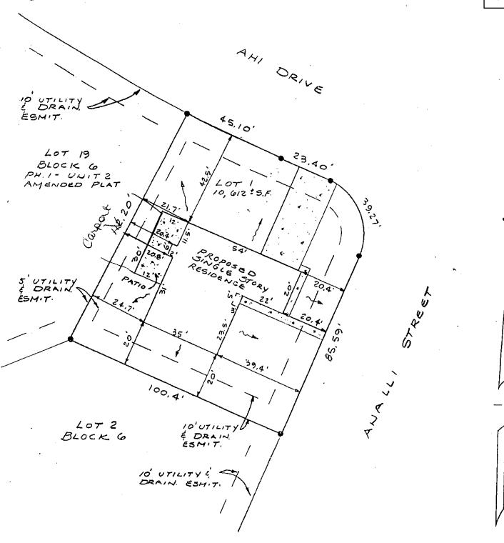
PLOT PLAN OF LOT 1- BLOCK 6 DIAMONDHEAD UNIT 10- PHASE 2 HANCOCK COUNTY, MS. FOR: GLENN SCHAUFFE
