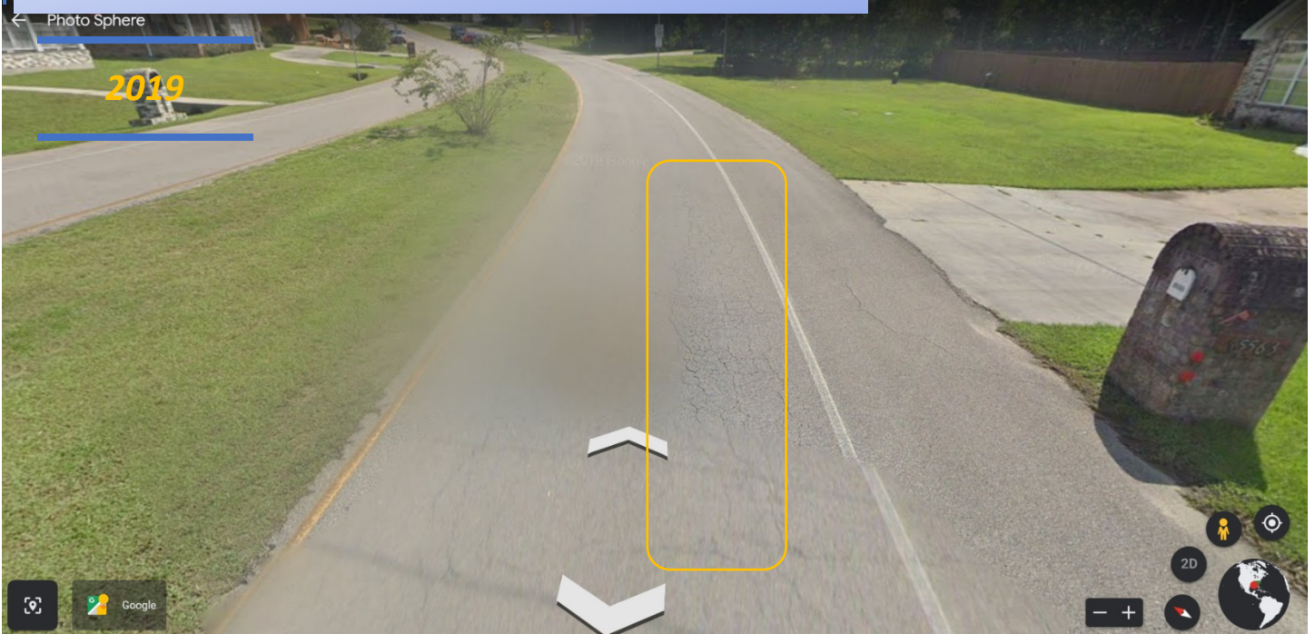
There is significant mass cracking and fatigue cracking along the area between Bayou Drive and 85553 DH Drive West. However, these issues were present in 2019 as indicated in the rectangular areas.
