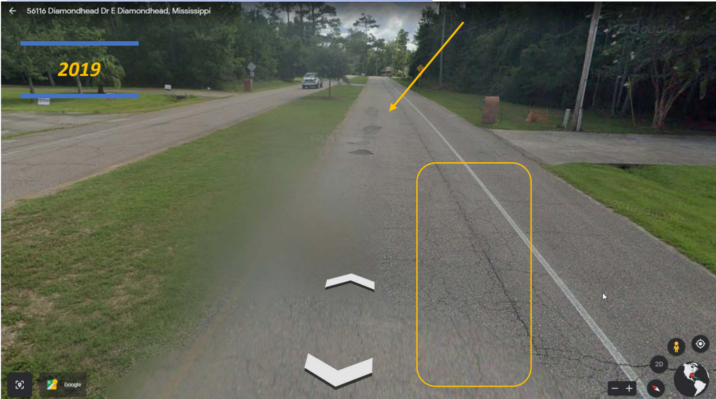
These distresses, potholes, mass cracking, transverse and block cracking, are visible in current and 2019 imagery in the same locations and general severity.
