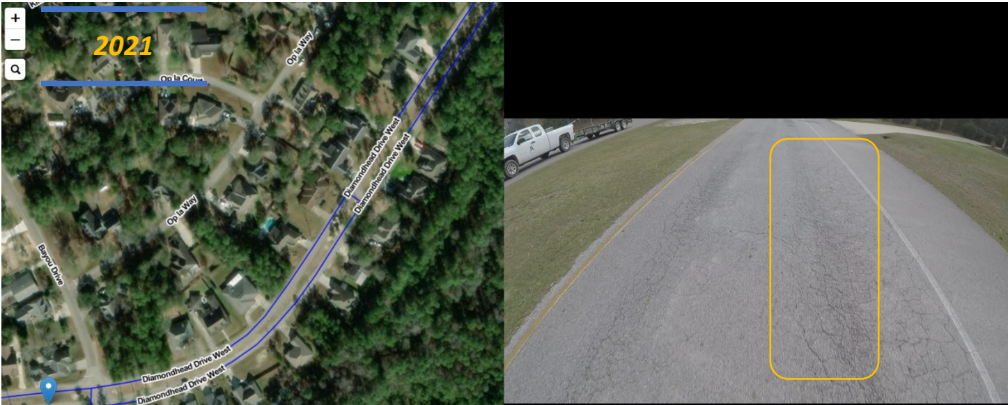
Severe shoving and fatigue cracking at the intersection of Bayou Drive and Diamondhead Drive West in past imagery and present.
