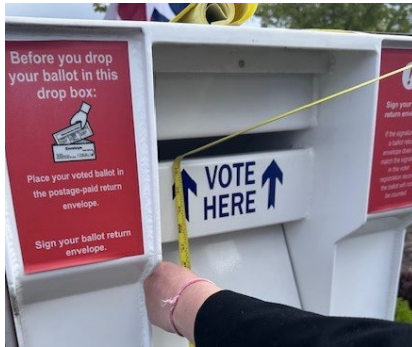
Figure VII: Photos of drop boxes with openings above 48" and gaps wider than ½"
