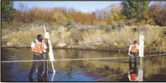
These scientists are measuring the flow of ground water into the Little Deschutes River through the streambed.
