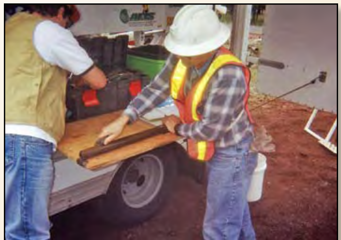
Geologists examined drill-core samples to define the geology at different depths.
