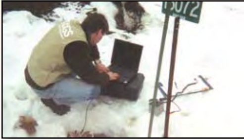
The USGS measured water levels in the aquifer under the La Pine area to determine the direction of ground-water flow.
