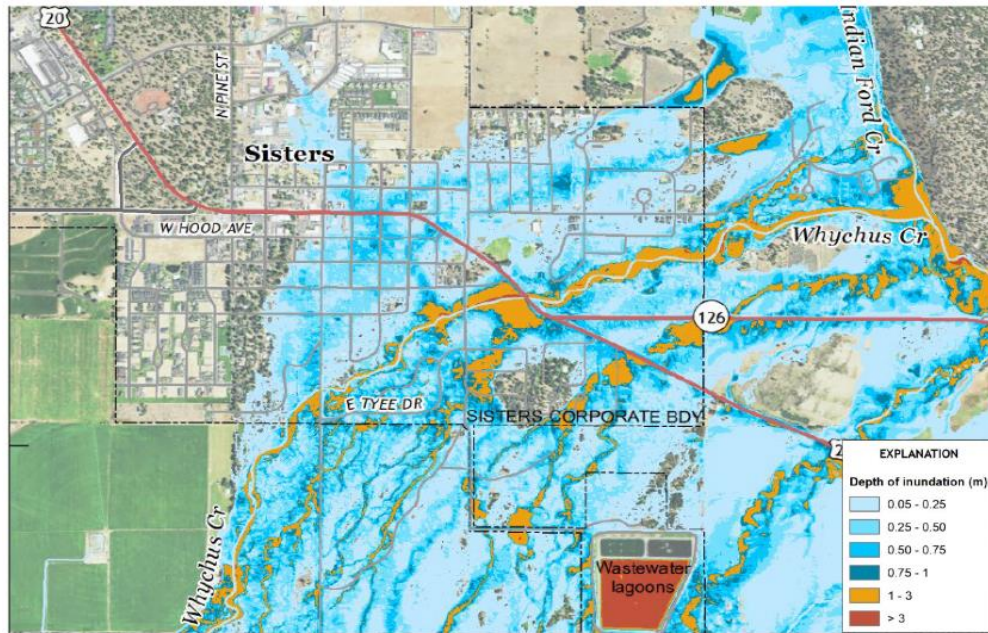
Figure SA-5 USGS 2-dimensional modeling results for flooding triggered by a hypothetical landslide of off South Sister landing in Carver Lake and evacuating all of its contents
