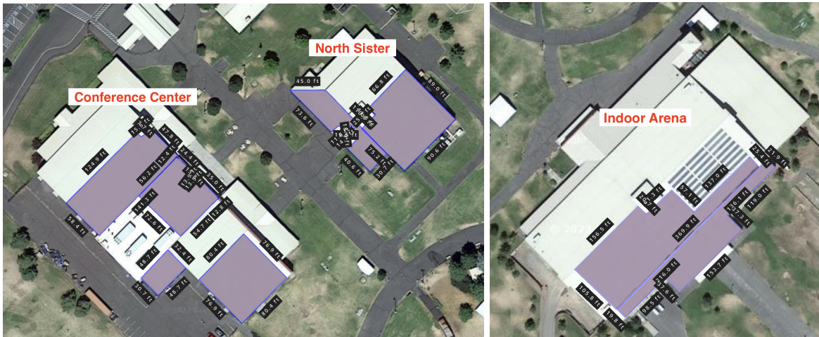
Figure 2. Available roof space with suitable PV tilt and azimuth; purple areas indicate possible PV locations
