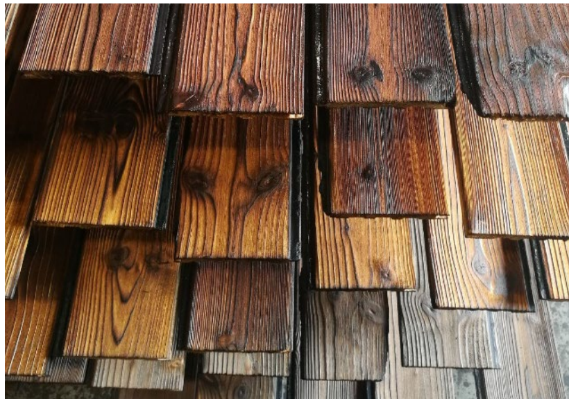
Figure 7: Example of shou sugi ban treated wood which can give the appearance of oiled, weathered wood cladding as recommended in the Western Design Theme.
