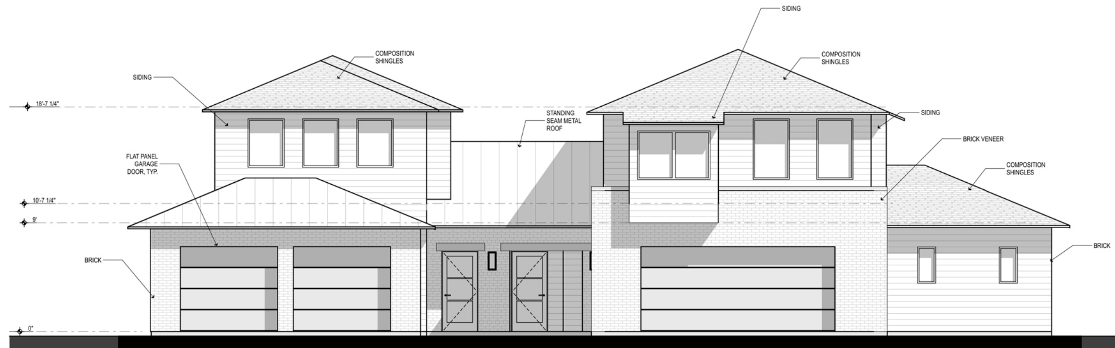
1 BUILDING E : FRONT ELEVATION SCALE: 1/4" = 1'-0"
