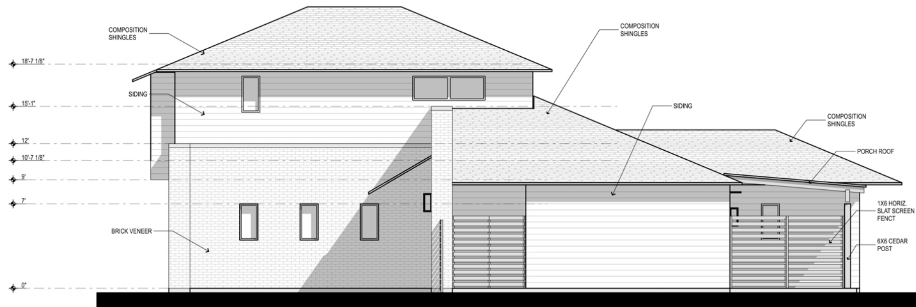
1 BUILDING C2 : RIGHT ELEVATION SCALE: 1/4" = 1'-0"
