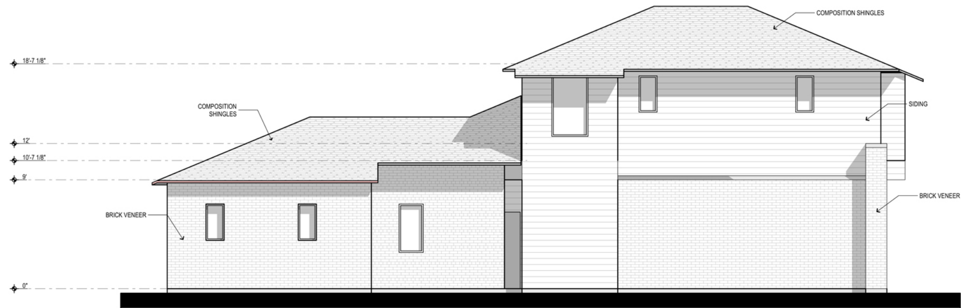
2 BUILDING C2 : LEFT ELEVATION SCALE: 1/4" = 1'-0"
