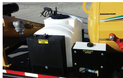
40 GALLON WATER TANK. Has 40 gal (151 L) of fresh water with 4 gpm (15 L/min) @ 3,000 psi water pump.
