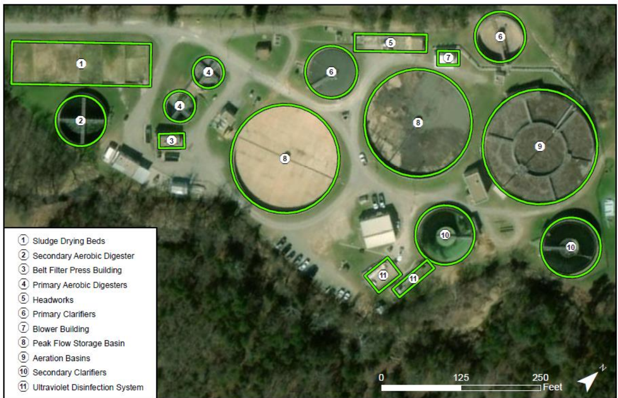
Figure 2-5: Paw Paw Wastewater Treatment Plant Site Plan
