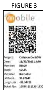
FIGURE 3 Paper tickets are created with encrypted QR code to transmit information/data.
