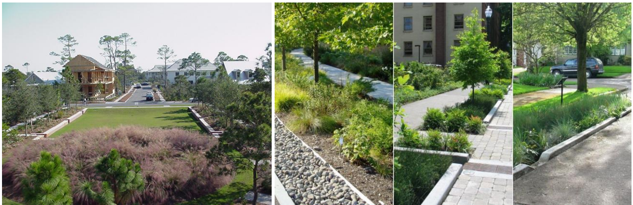
Figure 5 - 50: Alternative Stormwater Detention/Retention Facilities
