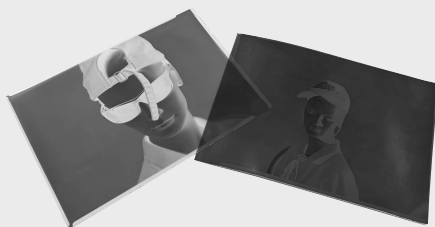
At left, a 5x7 film processed into a negative. At right, a 5x7 sheet of printing paper used to check for light leaks in the camera.
