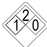
ALERTING SIGN (FOR DIESEL FUEL)
