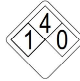
ALERTING SIGN (FOR PROPANE)
