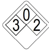
ALERTING SIGN (FOR CELL SITE BATTERIES)
