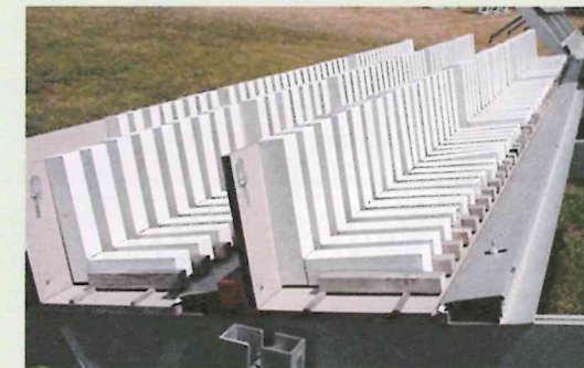
"L-Joint" visual appearance environmental test
