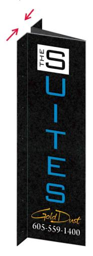
Exploded view. Sign will have 90 degree angle from mounting flanges to projecting portion of sign
