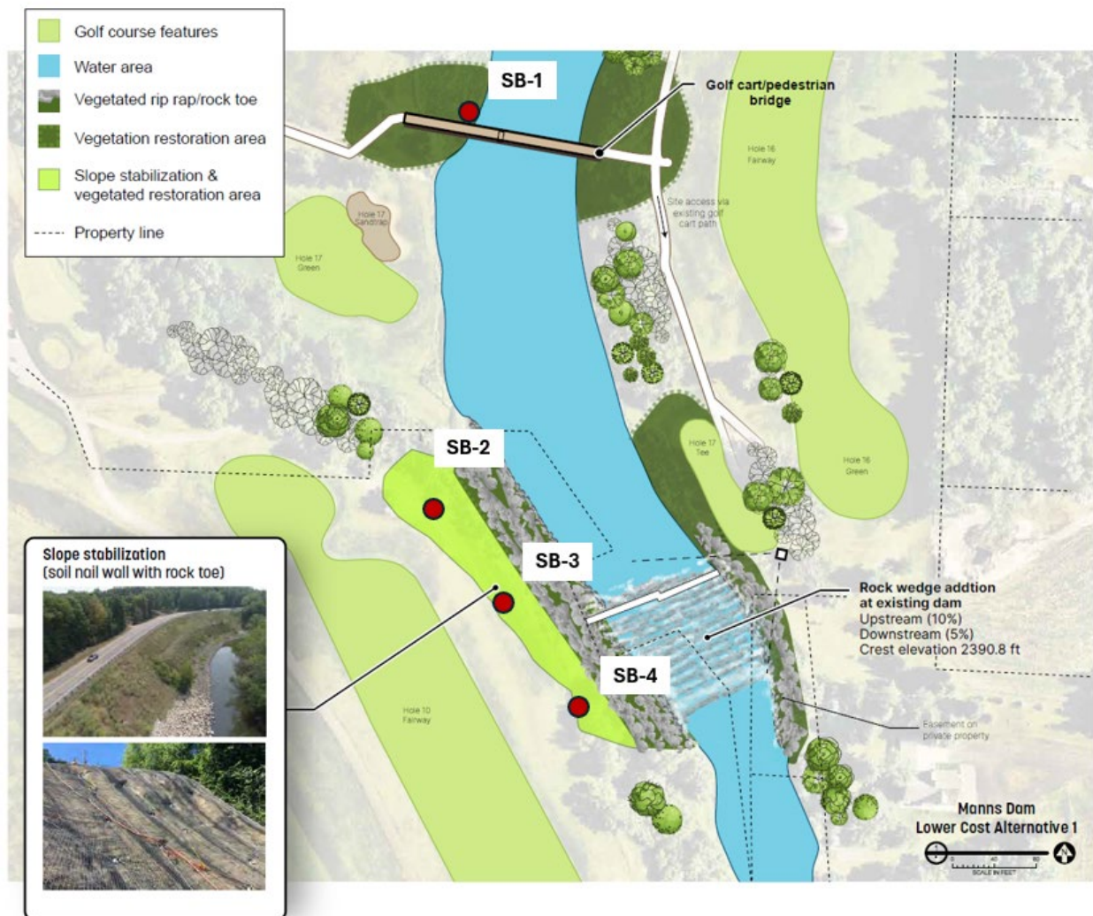
Figure 1 Planned geotechnical boring locations shown in red.
