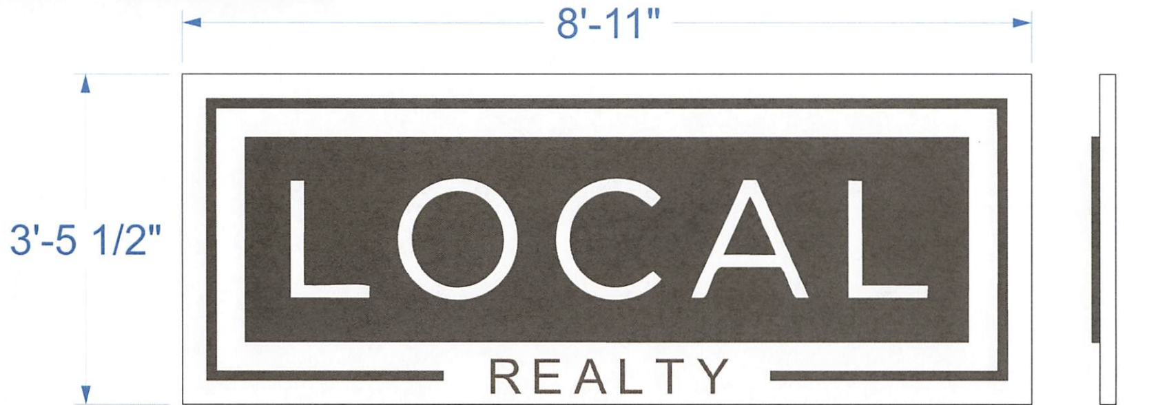
Fabricated aluminum pan sign with 2" returns with vinyl copy reading "REALTY", and inset line. Fabricated aluminum pan sign with vinyl overlays reading "LOCAL"
