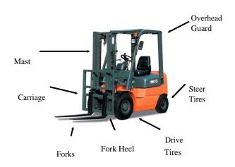
The main parts of a forklift are:
