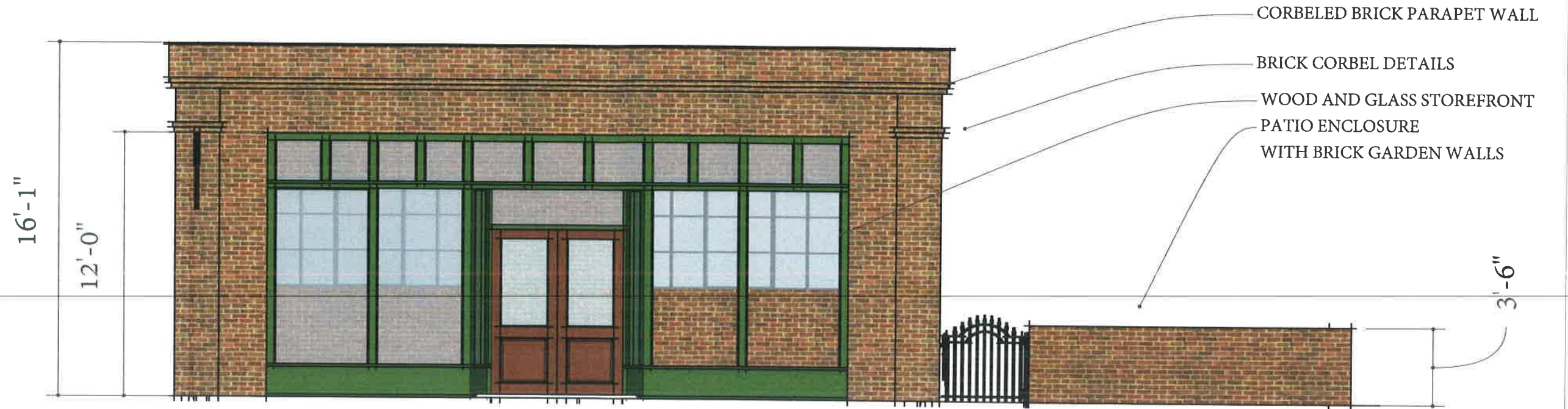
WEST ELEVATION FACING GILMER STREET
