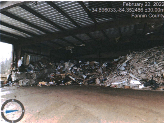
Photo Number: 3 of 4 Date: 2/22/2022 Time: 11:00 AM Weather: overcast Location: Sugar Creek C&D Transfer Station County: Fannin Photographer: Jason Rogers Observations: No partitioning between municipal waste (left side) and C&D waste (right side)
