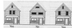
Façade openings are important in relative size and orientation, note the incompatible building.
