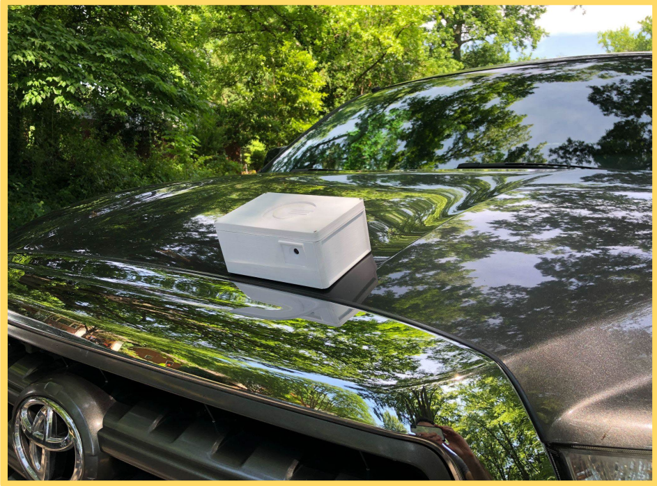
1. Battery-powered “Roadie” mounts magnetically to the hood of any vehicle
