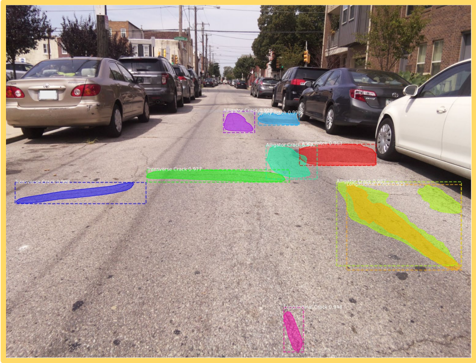
3. AI imagery output that is reviewed as part of the QA process.
