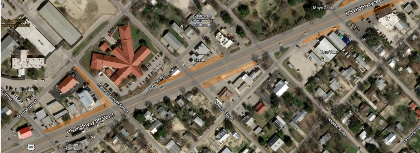
Parking Control: The images above show example application areas of parking control and management. Reconfiguring block-length access points into single or multiple driveways allows for greater delineation between spaces and increases safety for all modes. The areas highlighted in orange indicate where parking control could be implemented along Highway 90.
