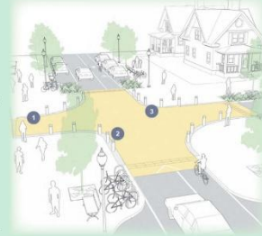
RAISED INTERSECTION Drawing sourced from NACTO
