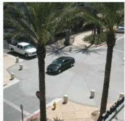
Curbless intersection with protective bollards
