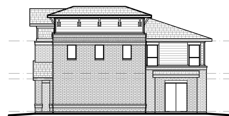
4 | BUILDING 3 AND 4 - EAST ELEVATION SC: 1/16" = 1'-0"
