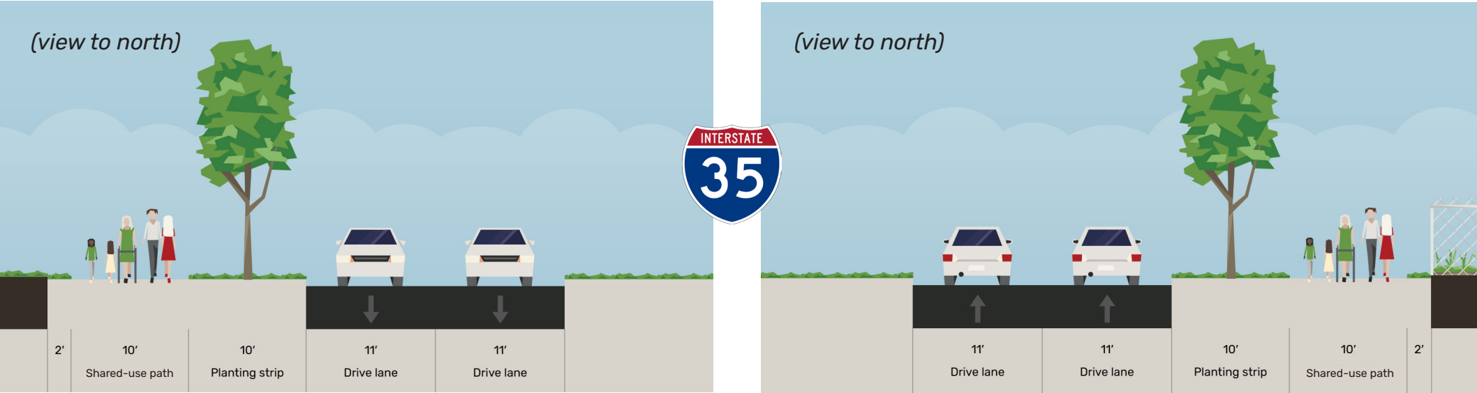
Exhibit 107. Proposed Typical Cross-Section on S. Stemmons Freeway (290' ROW)
