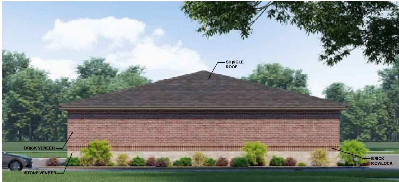
GARAGE W/ STORAGE - SIDE ELEVATION
