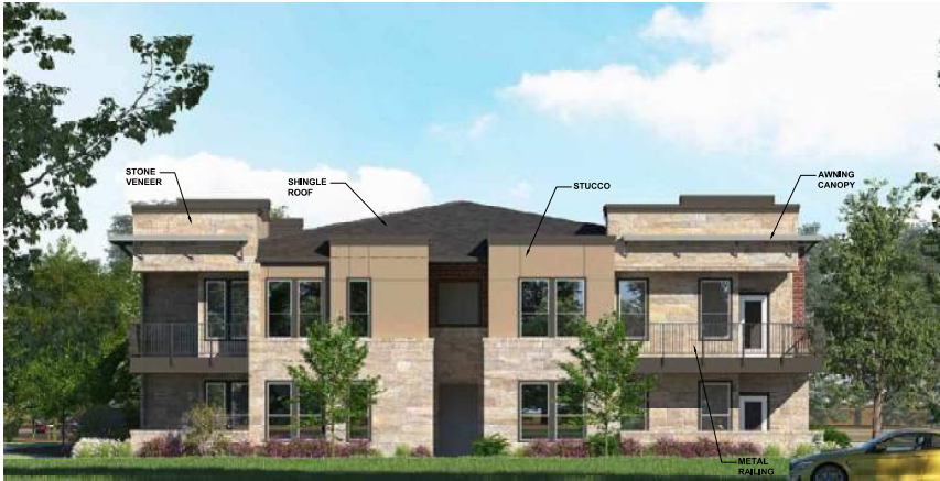
BLDG 'C' - LEFT ELEVATION
