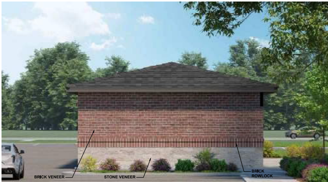
TYPICAL GARAGE - SIDE ELEVATION
