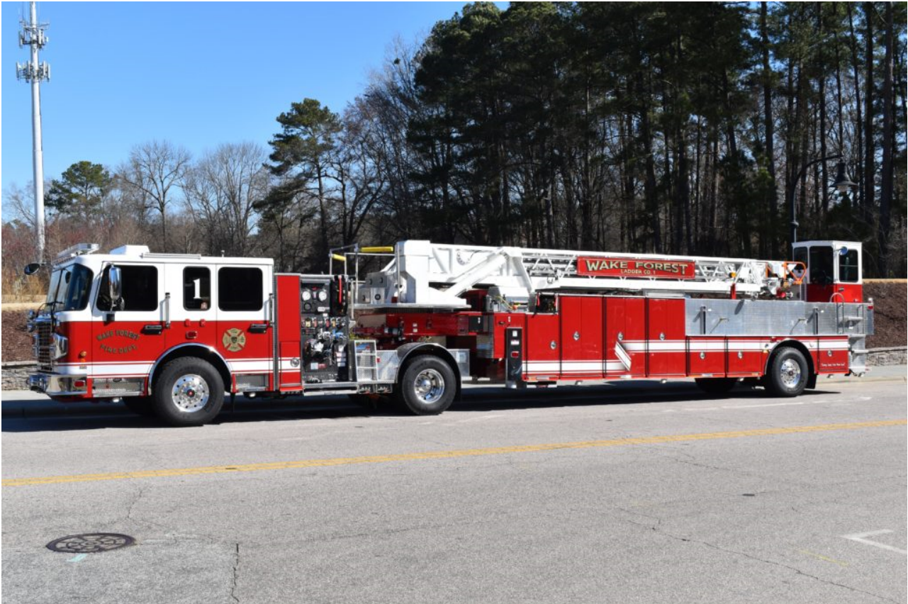
Spartan ER built this 105-foot Tractor Drawn Aerial (TDA) quint, known as a
