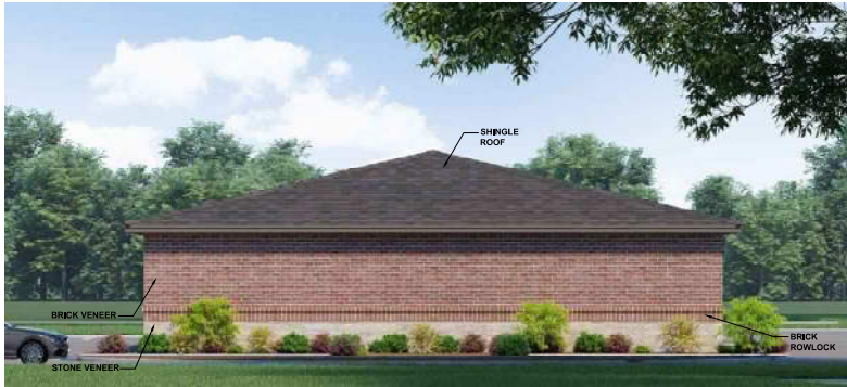
GARAGE W/ STORAGE - SIDE ELEVATION
