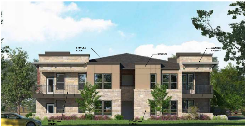
BLDG 'C' - RIGHT ELEVATION
