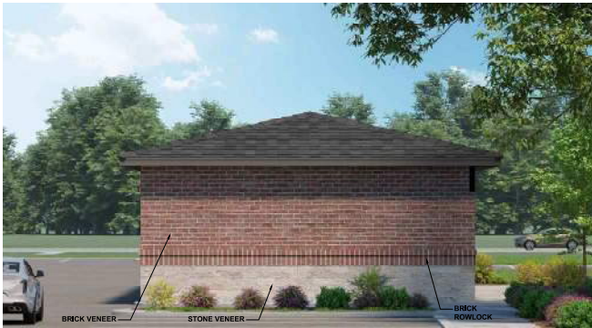
TYPICAL GARAGE - SIDE ELEVATION
