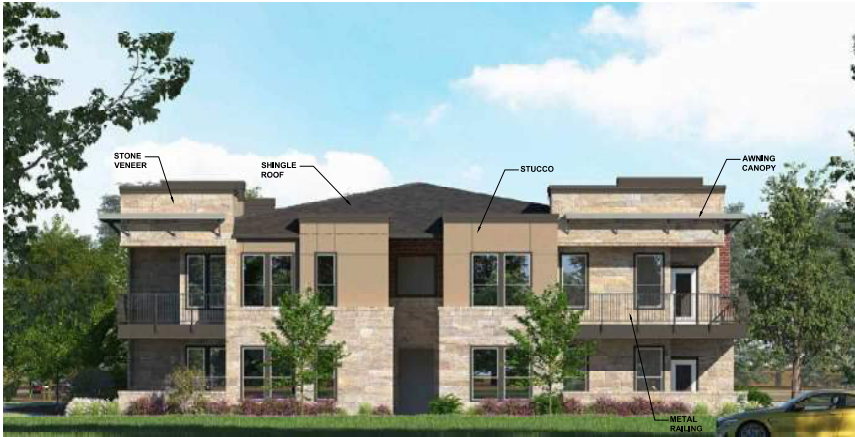
BLDG 'C' - LEFT ELEVATION
