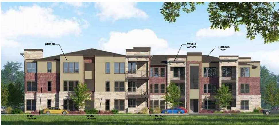
BLDG 'A' - RIGHT ELEVATION FRONTING INTERIOR STREET
