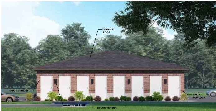
GARAGE W/ STORAGE - SIDE ELEVATION (STORAGES)
