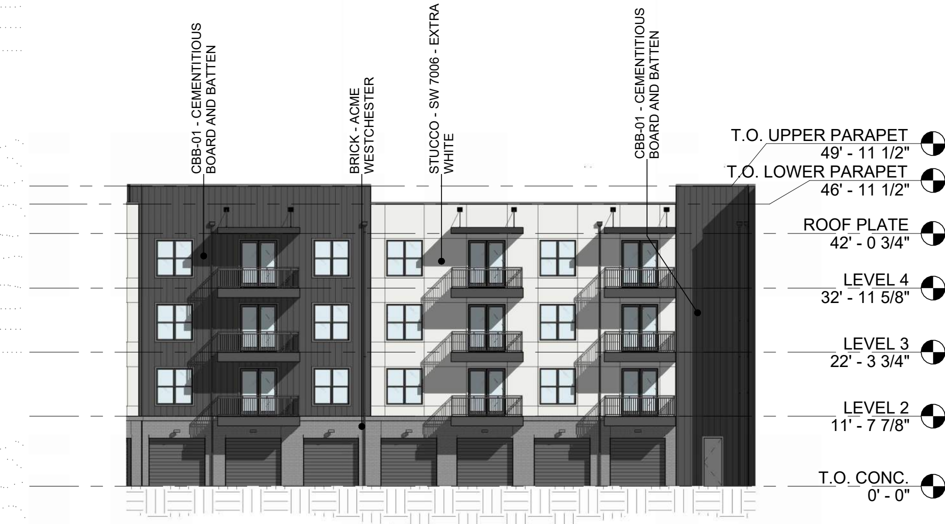
2 Building II - Elevation - Courtyard Northeast 1/16" = 1'-0"
