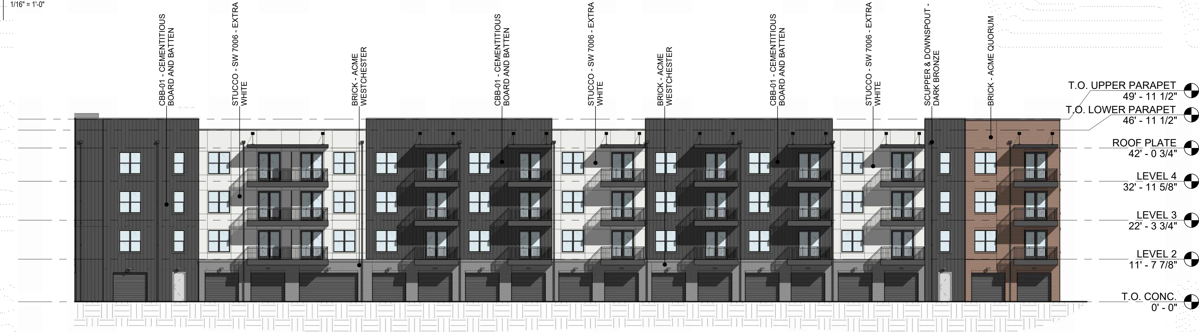
2 Building II - Elevation - Courtyard Northeast 1/16" = 1'-0"
