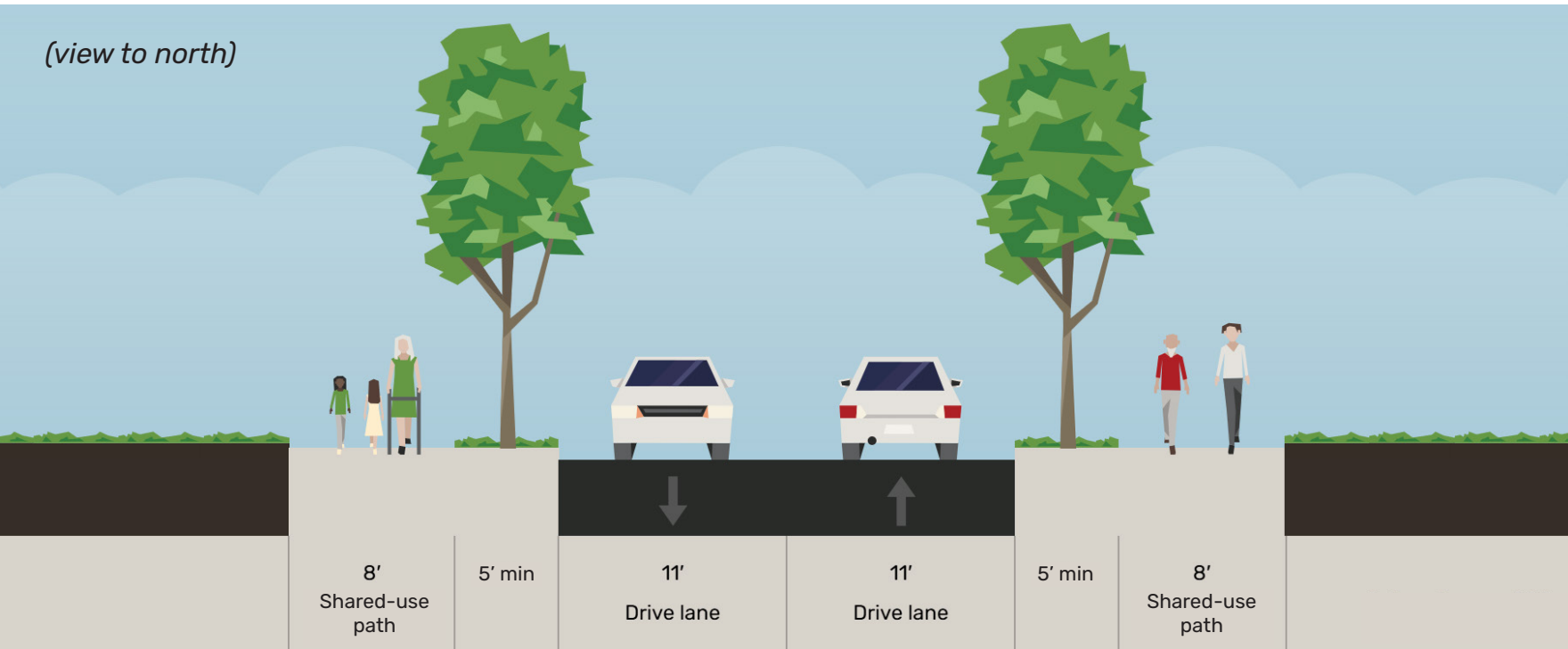
Exhibit 101. Proposed Typical Cross-Section on Garrison Road (North of Cliff Oaks Drive) (60' ROW min)
