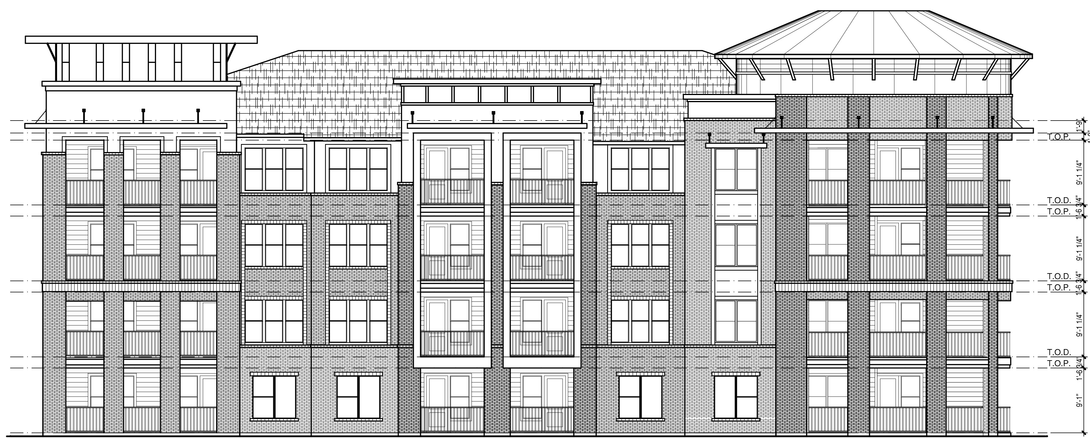
1 BUILDING B SIDE ELEVATION (WEST) SCALE: 1/8" = 1'-0"
