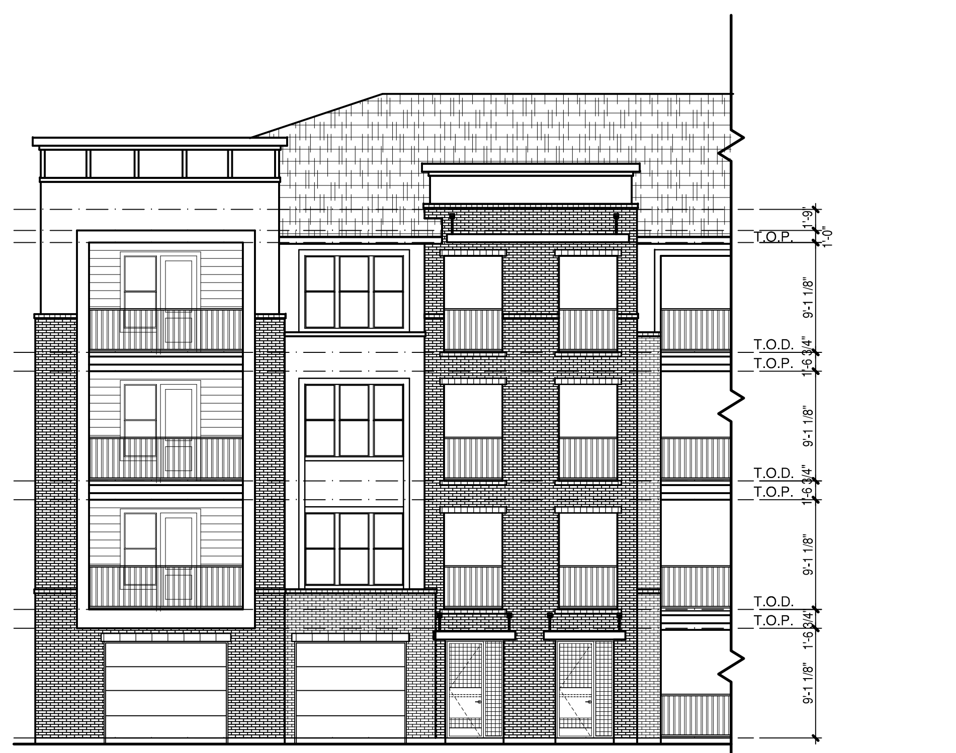
1 BUILDING C REAR ELEVATION (WEST) SCALE: 1/8" = 1'-0"
