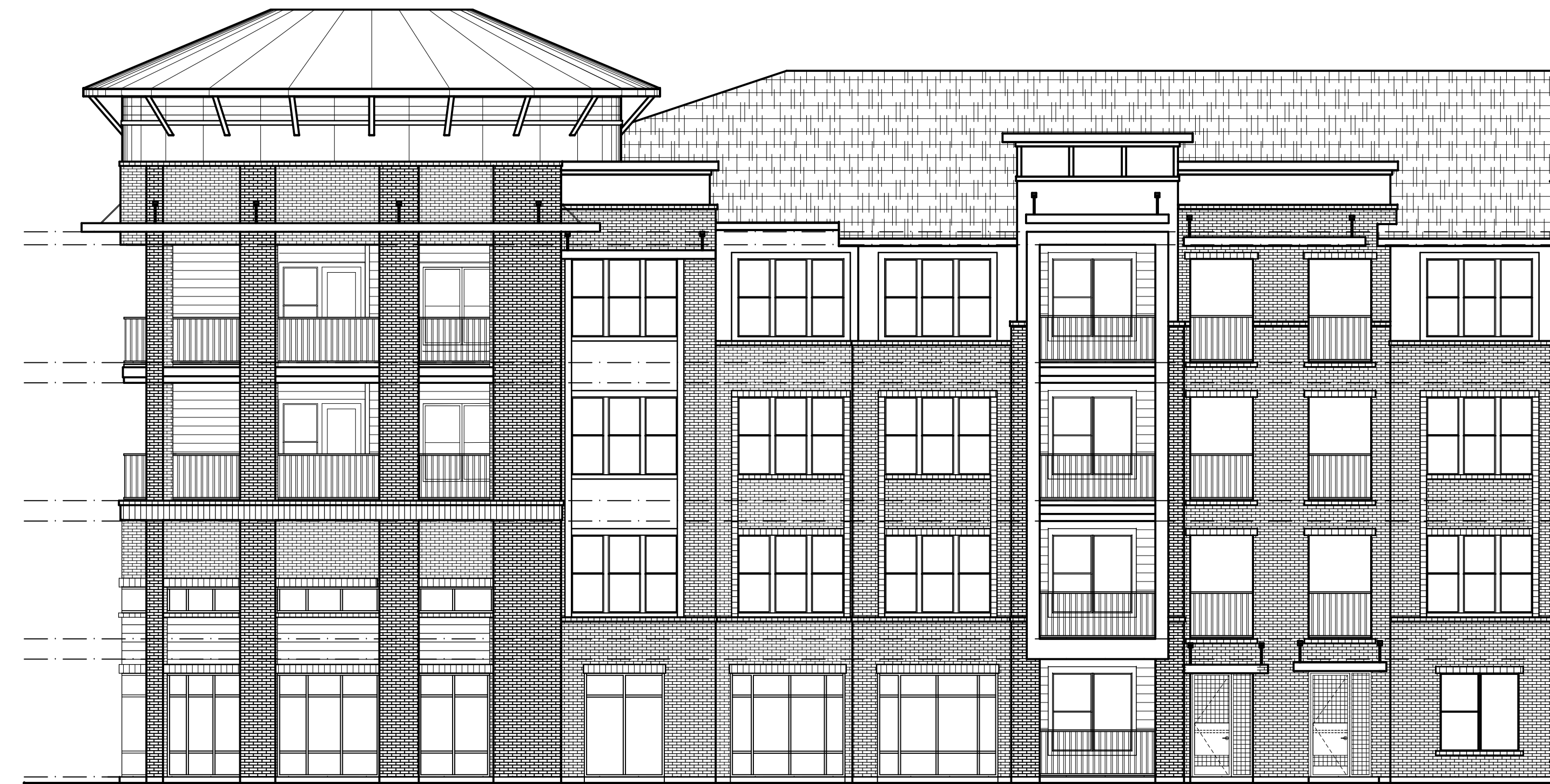
1b BUILDING A FRONT ELEVATION (SOUTH) SCALE: 1/8" = 1'-0"
