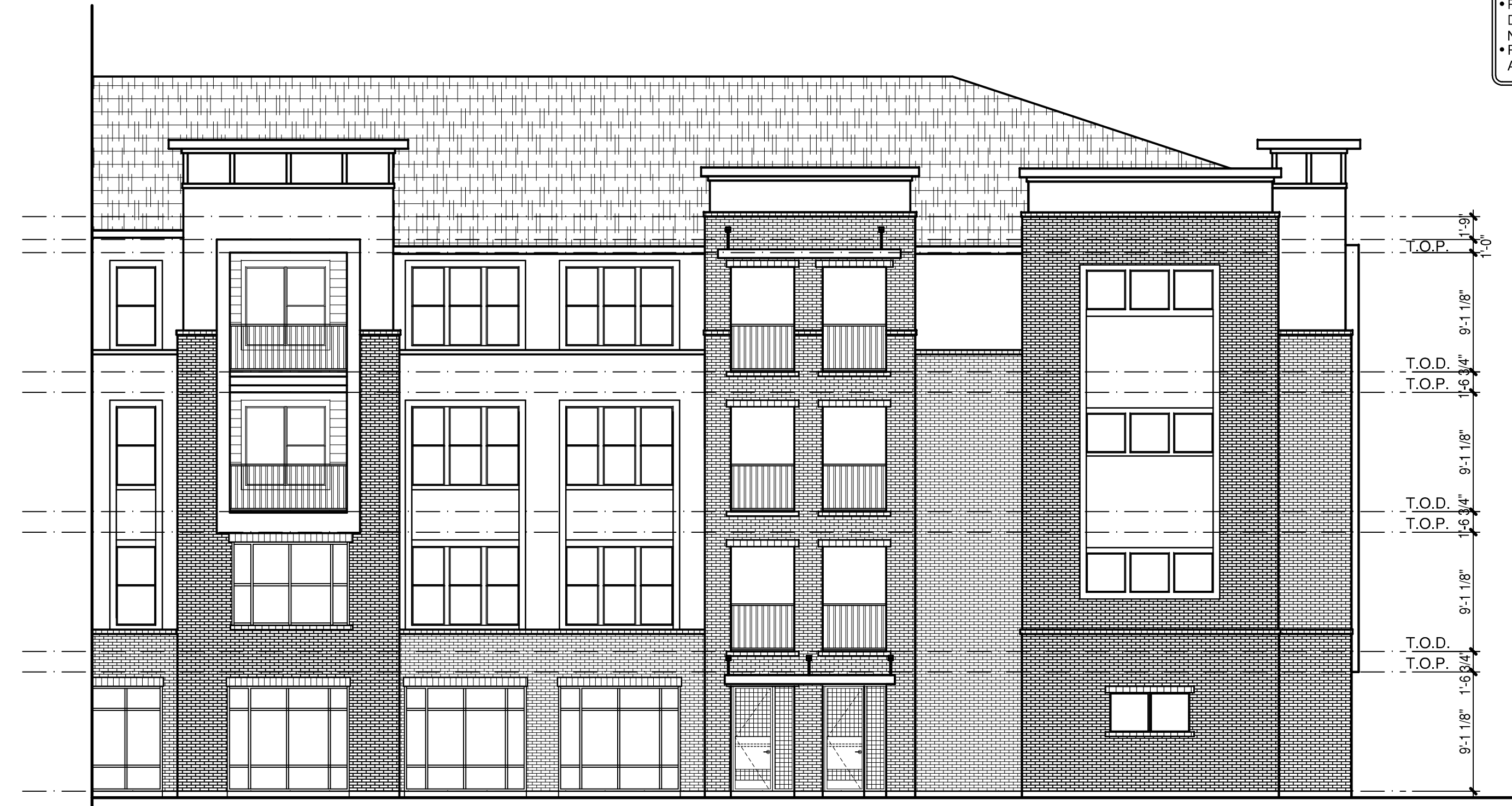
2 BUILDING A REAR ELEVATION (EAST) SCALE: 1/8" = 1'-0"
