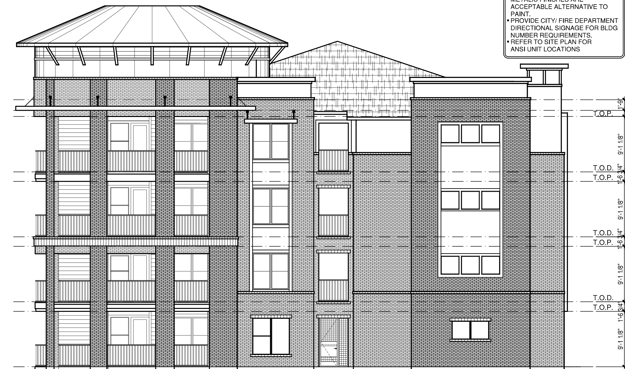
3 BUILDING C FRONT ELEVATION (NORTH) SCALE: 1/8" = 1'-0"
