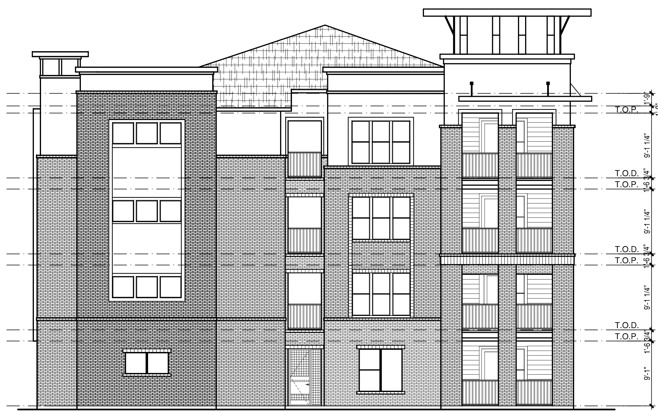
3 BUILDING B SIDE ELEVATION SCALE: 1/8" = 1'-0"
