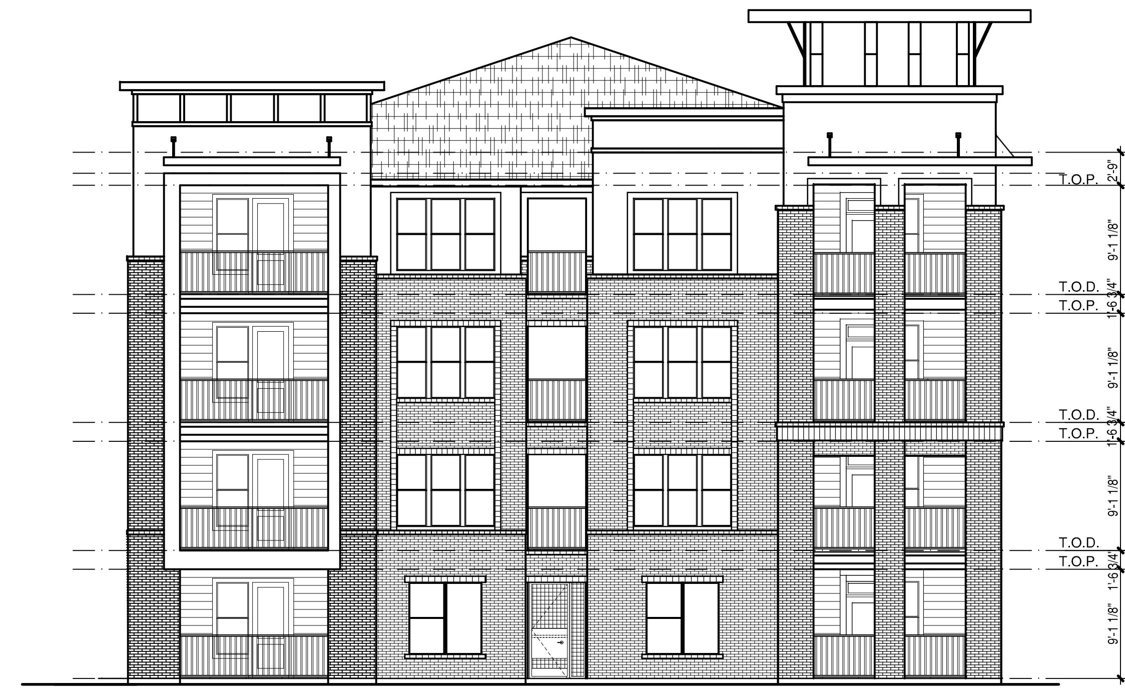
3 BUILDING A SIDE ELEVATION (NORTH) SCALE: 1/8" = 1'-0"
