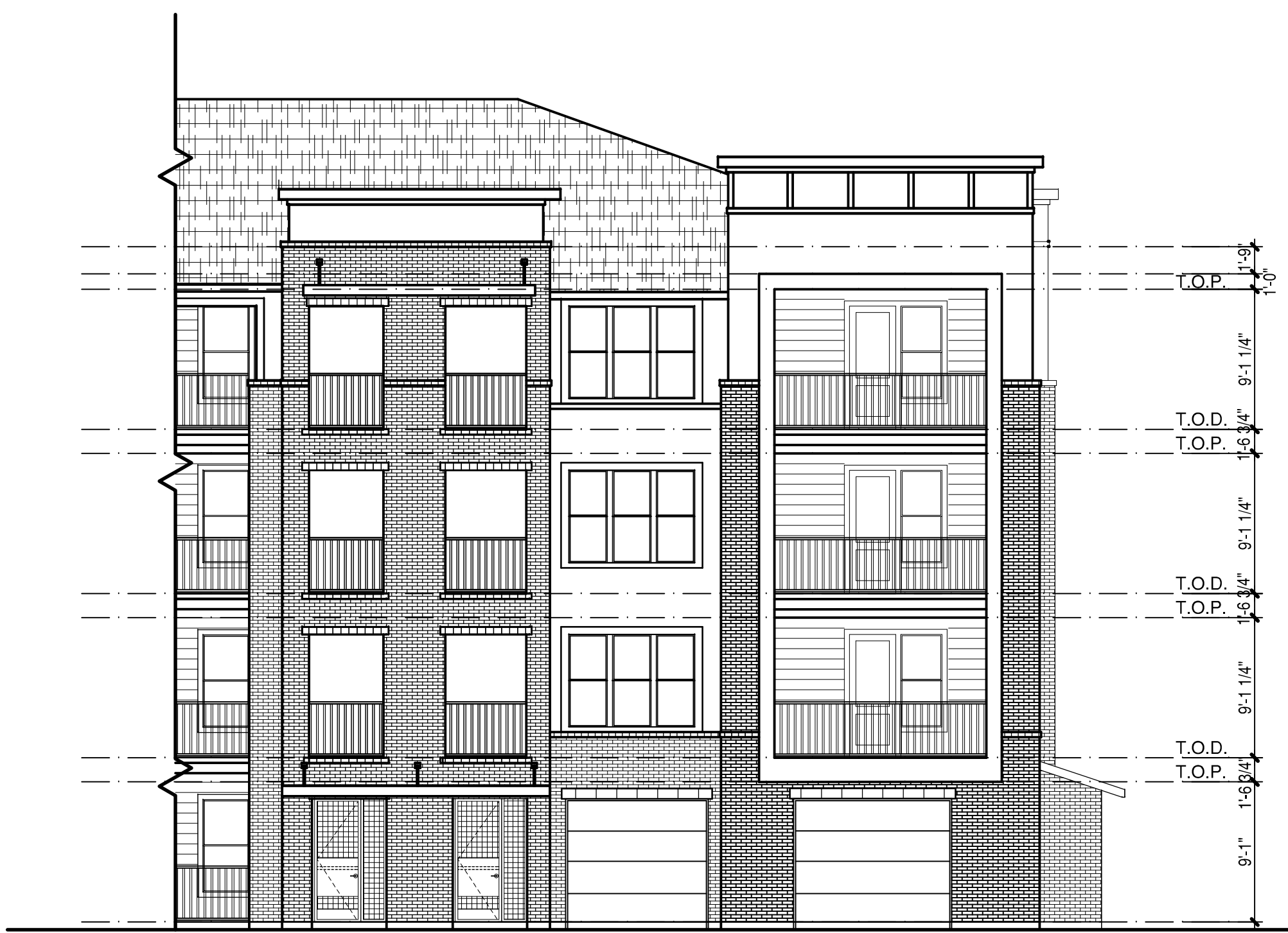
2 BUILDING B REAR ELEVATION SCALE: 1/8" = 1'-0"
