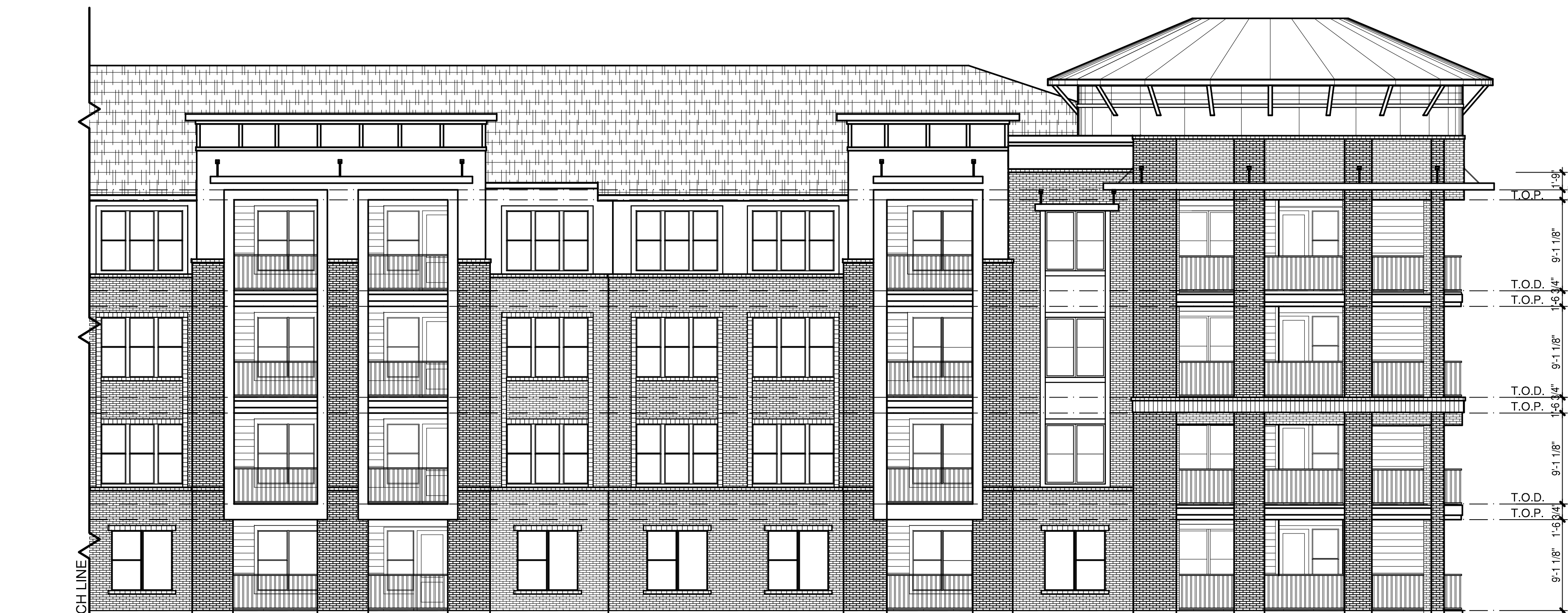
1a BUILDING A FRONT ELEVATION (SOUTH) SCALE: 1/8" = 1'-0"
