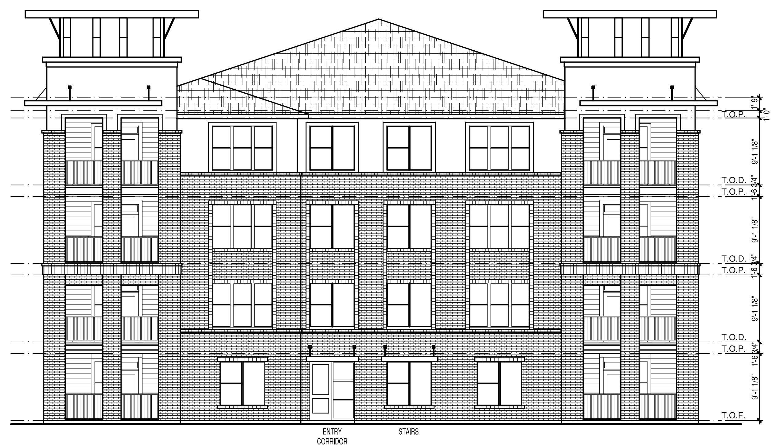
2 BUILDING D ELEVATION (SOUTH) SCALE: 1/8" = 1'-0"
