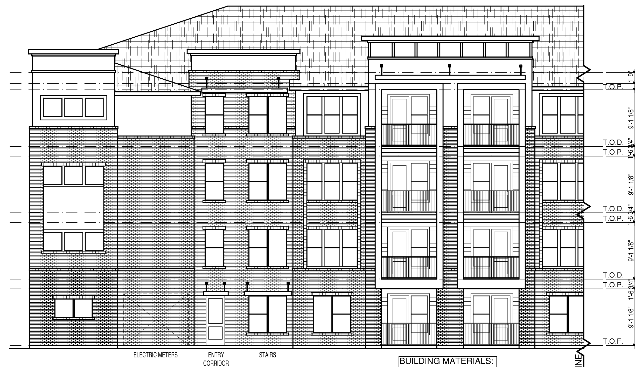
1a BUILDING D ELEVATION (WEST) SCALE: 1/8" = 1'-0"
