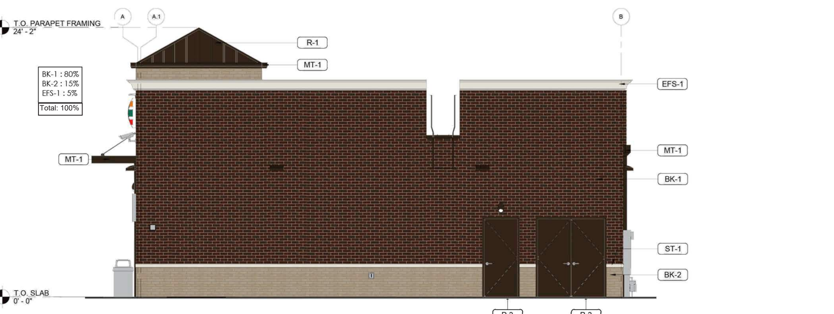
3 ELEVATION - RIGHT SIDE 3/16" = 1'-0"
