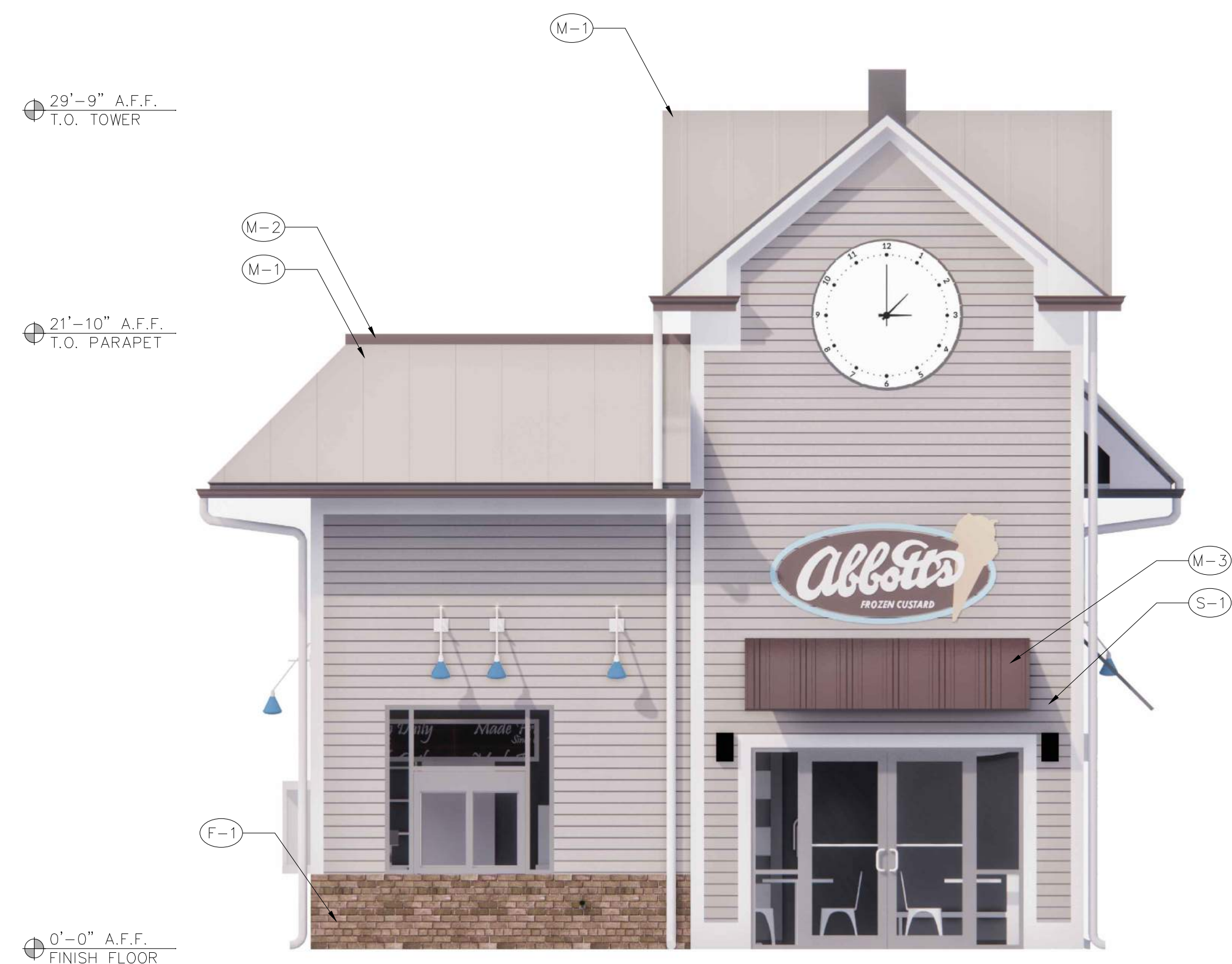
1 EXTERIOR ELEVATION- EAST SCALE: 1/4" = 1'-0"
