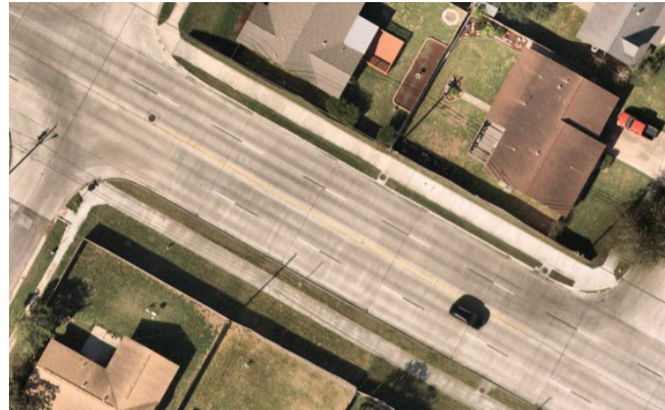
Shared-use path on both sides of Williams Drive in Corpus Christi, Texas
