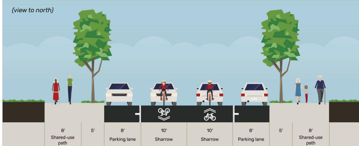
Exhibit 86. Proposed Typical Cross-Section on North Corinth Street (62' ROW)
