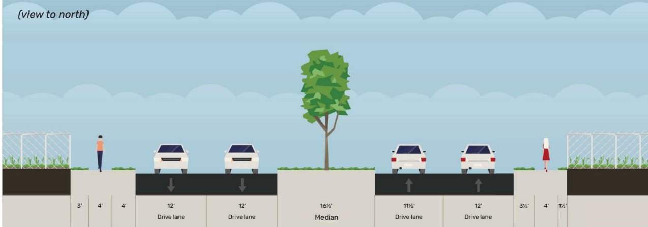
Exhibit 64. Proposed Typical Cross-Section on Corinth Parkway (Creek Bend Drive to IH 35 @ Lake Sharon Drive) (84' ROW)
