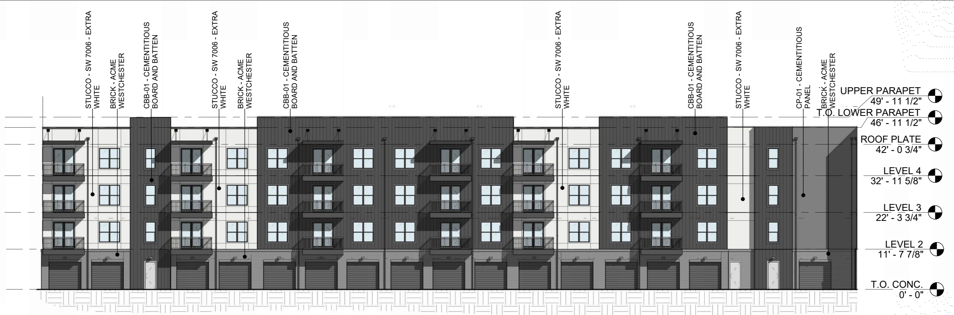
3 Building I - Elevation - Courtyard South 1/16" = 1'-0"
