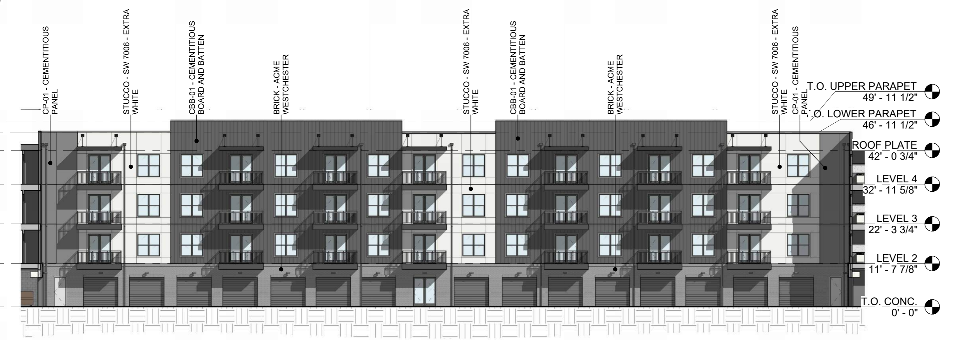
2 Building I - Elevation - Courtyard West 1/16" = 1'-0"
