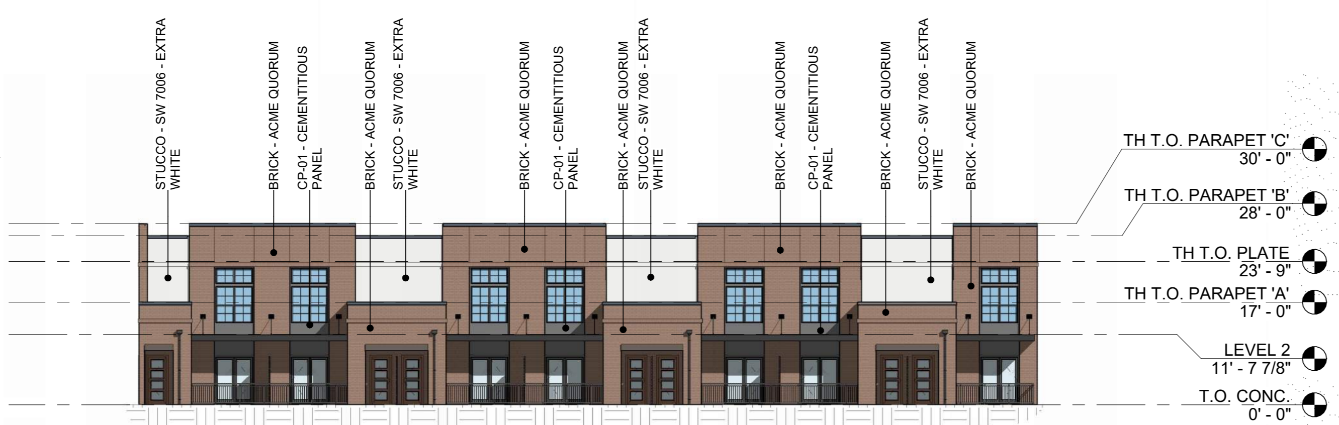
1 Building IV - Elevation - North 1/16" = 1'-0"
