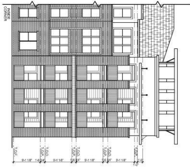
1 BUILDING D ELEVATION (WEST) SCALE: 1/8" = 1'-0"
